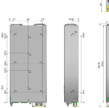
(\*) M3 threaded hole. Maximum screw depth: 3mm
