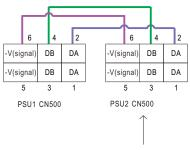
If the lines of CN500 are too long, they should be twisted in pairs to avoid the noise.
