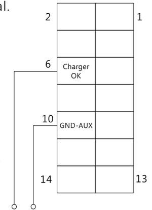
5.2.5 Battery OK signal(NPB/NPP-450/750/1200/1700)
