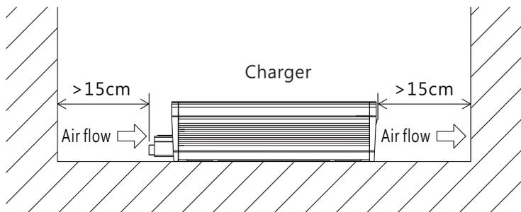
Figure 3-1 set-up recommendation
