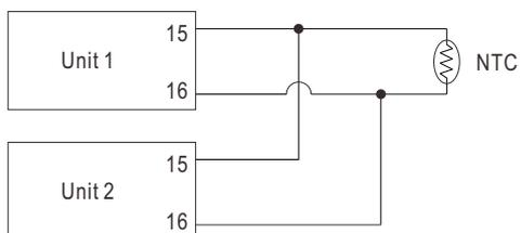
When multiple chargers are connected in parallel, please configure with the NTC as exhibited in the diagram .
