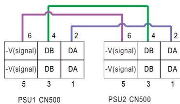
If the lines of CN500 are too long, they should be twisted in pairs to avoid the noise.
