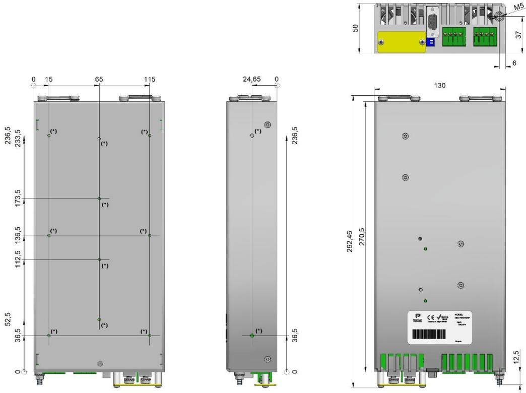
(\*) M3 threaded hole. Maximum screw depth: 3mm
