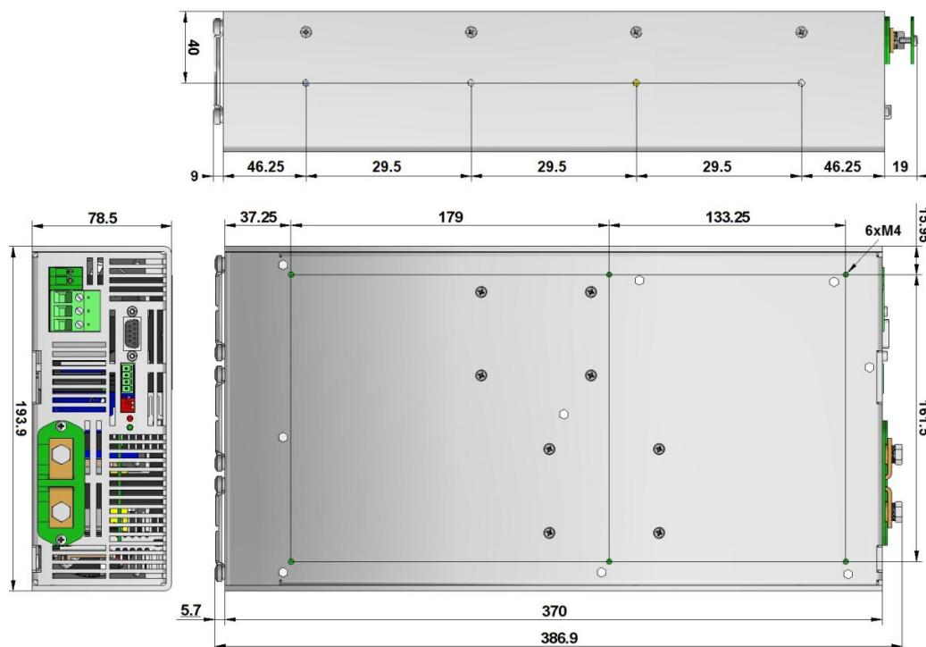
Maximum depth for the screws M4: 4.5mm
