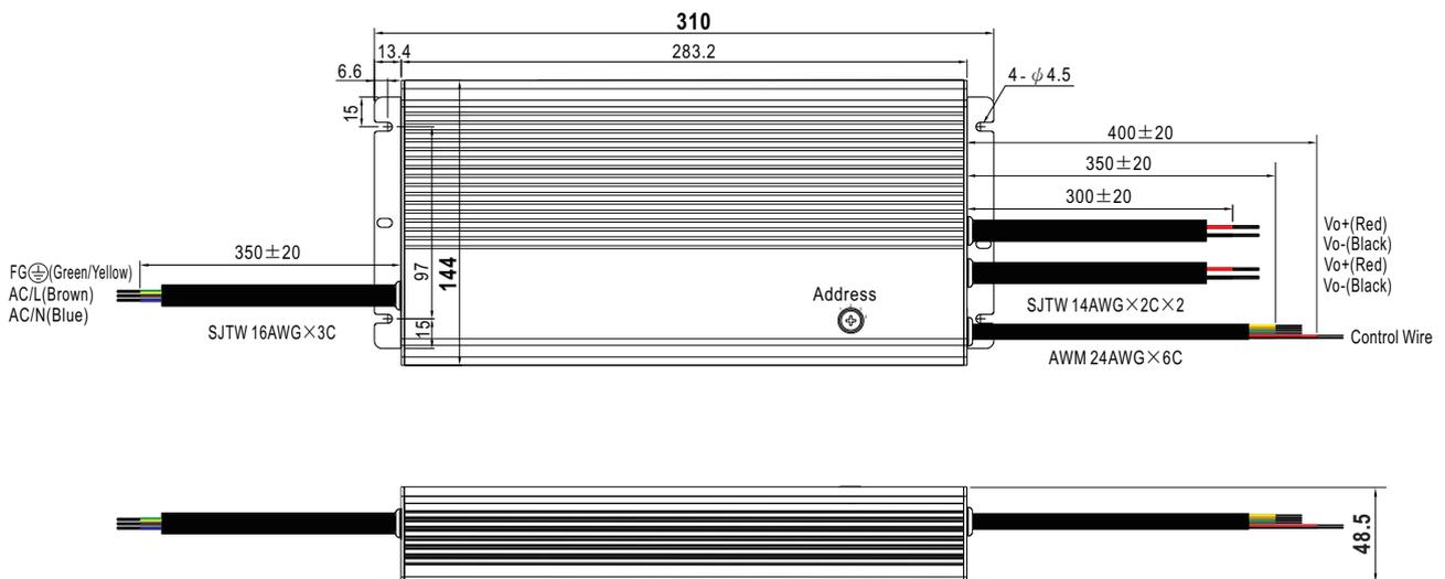
※ Output voltage current level can be adjusted through internal potentiometer.
