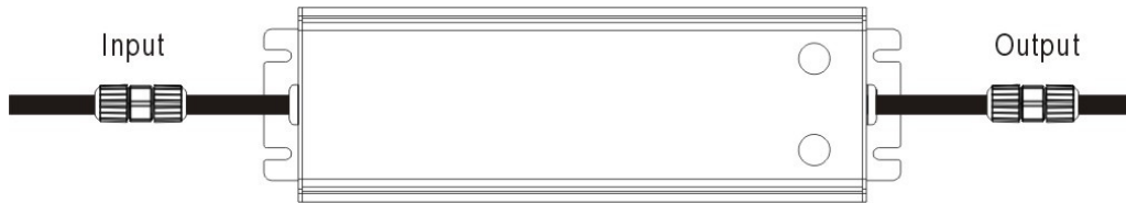
Fig.4.12 Setup diagram of LED power supply with waterproof connectors
